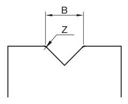
To simulate the Rolla-V on a machine graphical input, use a v-width of **B** and v-corner radius of **Z**.
